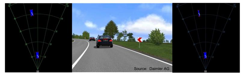
has been used commonly for controlability studies of ADAS systems in *Driver in the loop* simulations, for example in order to generate a warning tone and emergency braking functions used in order to evaluate the basic function of a vehicle in **complex traffic situations**, including effects resulting from the geometrical position of **several contributing sensors**
