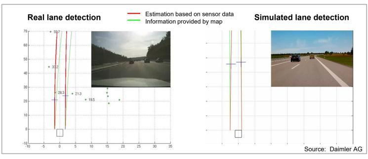
used to verify the ability of the environmental perception software to handle **imperfect sensor input** and to take advantage from the knowledge about different sensor properties in **sensor fusion**; evaluate, under which sensor conditions the fusion reaches its **functional limits**. **Parameters** describing the stochastic distribution depend on
