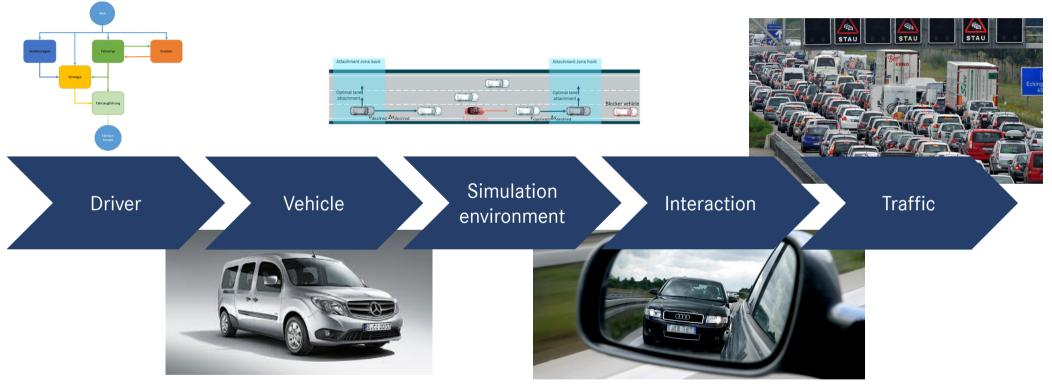
Realistic traffic flow results from interaction of various driver types in vehicles with different performance
